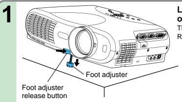
Lift the front of the projector until the desired tilt angle is obtained and hold down the foot adjuster release button.
